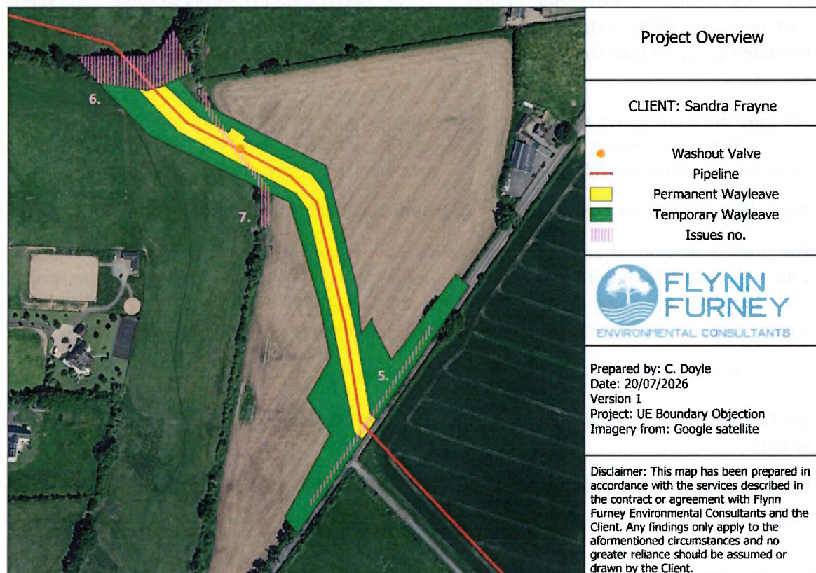
Figure 1: Overview of the area of interest, showing the proposed wayleaves, pipeline route and washout valve, along with the areas of interest of this report, issues 5, 6 and 7.
